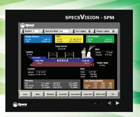
SPECSVISION-SPM is most useful and practical tool for monitoring, reporting and verification of CO<sub>2</sub> emissions and energy efficiency of all ships. It has following functions which can be adjusted based on the different ship types, sizes and operational profiles.
