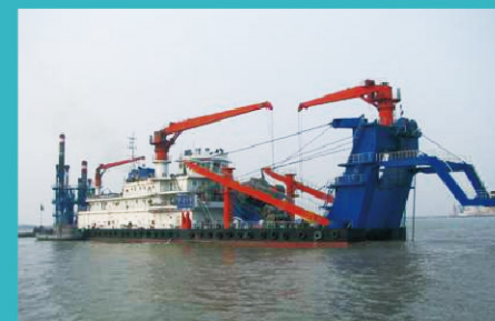
pic7 Lianyungang Port Group 3500m³/h Cutter Suction Dredger
