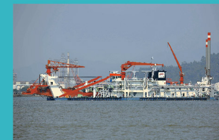
pic8 CRCC Harbor & Channel Engineering Bureau Group 5000m³/h Cutter Suction Dredger
