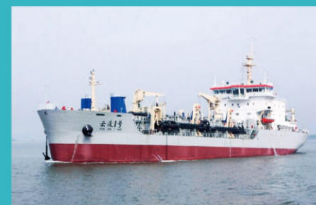
pic5 Lianyungang Port Group 5000m³/h Suction Hopper Dredger
