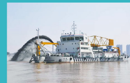
pic6 Changjiang Waterway Bureau 2000m³/h Suction Cupule Dredger
