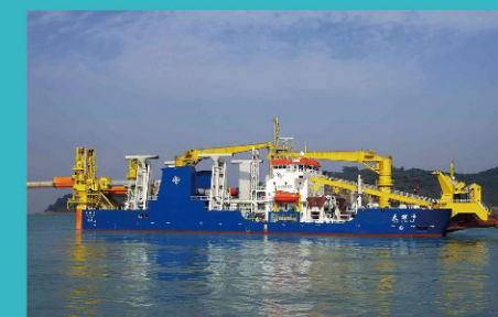
pic4 Tianjin Dredging Co.,Ltd 4500m³/h Cutter Suction Dredger
