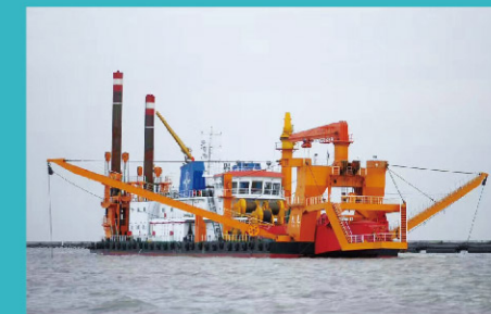
pic2 Tianjin Dredging Co.,Ltd 3000m³/h Cutter Suction Dredger
