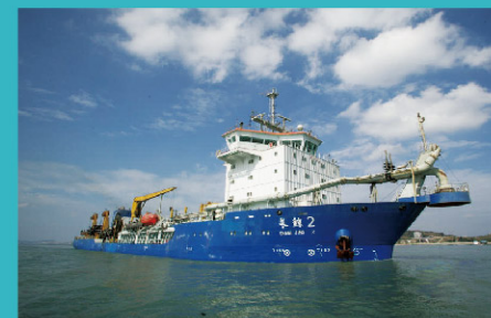
pic3 Changjiang Waterway Bureau 8000m³/h Suction Hopper Dredger
