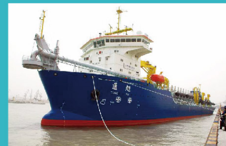
pic1 Tianjin Dredging Co.,Ltd 13000m³/h Large Suction Hopper Dredger
